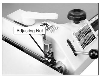
Figure 24. Aligning the round rail.
